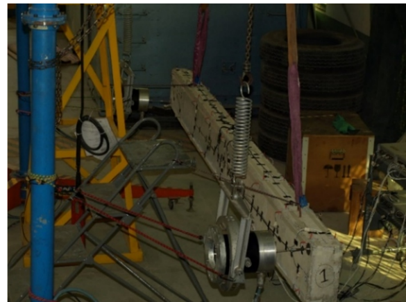
Fig. 4. Experimental Modal Testing arrangement with exciter support system
