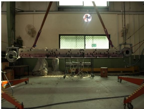
Fig. 5. Experimental Modal Testing arrangement with free-free boundary conditions
